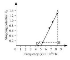
It can be observed that the obtained curve is a straight line. It intersects the v-axis at  $5 \times 10^{14}$  Hz, which is the threshold frequency (v<sub>0</sub>) of the material. Point D corresponds to a frequency less than the threshold frequency. Hence, there is no photoelectric emission for the  $\lambda_5$  line, and therefore, no stopping voltage is required to stop the current.
